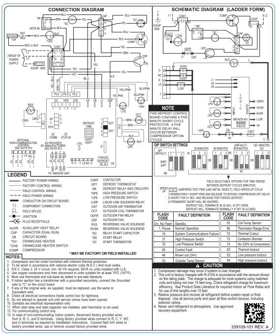
Fig. 1 - Wiring Diagram — Model size 1.5 - 5 tons, 208/230-1
