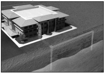
• Closed Loop/Ground Water Plate Heat Exchanger Systems utilize lake, ocean, well water or other water sources to maintain closed loop water temperatures in multi-unit LX Base systems. A plate frame heal exchanger isolates the units from any contaminating effects of the water source, and allows periodic cleaning of the heat exchanger during off peak hours.
