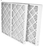
Standard supplied filter is a pleated MERV 4, 1 in. [2.54 cm]. An optional low static high efficiency 2 in. [5.1 cm] MERV 13, for LEED certification points, is also available.
