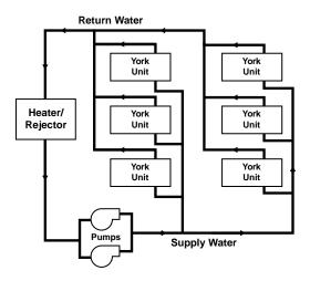
environment for all building areas. Excess heat can be stored for later utilization or be added or removed in one of three ways; by ground-source heat exchanger loops: plate heat exchangers connected to other water sources, or conventional cooler/boiler configurations. Your York representative has the expertise and computer software to assist in determining optimum system type for specific applications.
