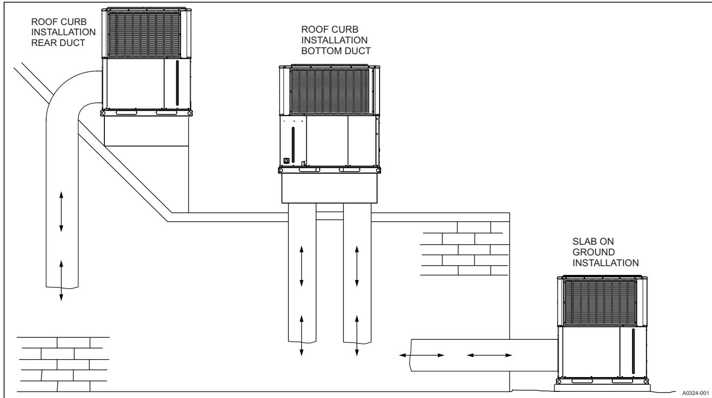
**UNIT TYPICAL SLAB ON GROUND INSTALLATION**
