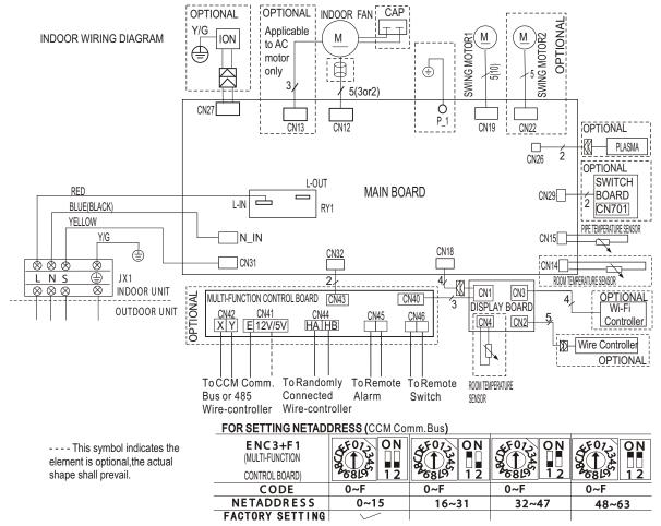
Fig. 9 – Wiring Diagram Sizes 09–12 (115V)
