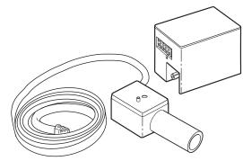
Fig. 1 – Condensate Pump Accessory
