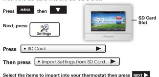
Your thermostat will automatically save your new photos and settings in it's internal memory. When finished, you may remove the SD card. It is not needed for normal thermostat operation.
