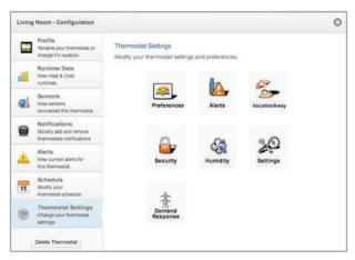
The Demand Response configuration page, shown below, is where the thermostat is configured to respond to the energy provider's signals. It also sets operational parameters for the thermostat.
