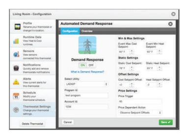
The right column of the ADR configuration page is where the occupant adjusts the operational parameters for ADR. The utility may send up to 3 types of ADR signals to Skyport. These are:
