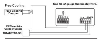
Free Cooling utilizes the Y1 terminal for the operation of 1st stage cooling. If mechanical (compressor) cooling is also present, the mechanical cooling is connected to the Y2 terminal in this instance.
