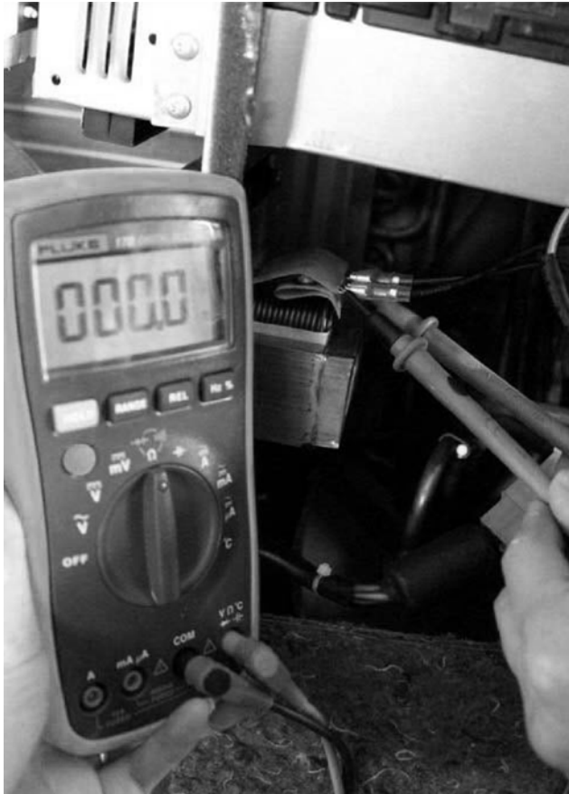
Fig. 22 – Reactor resistance test
