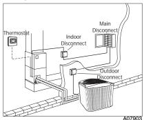
Fig. 1 - Electrical Disconnects
