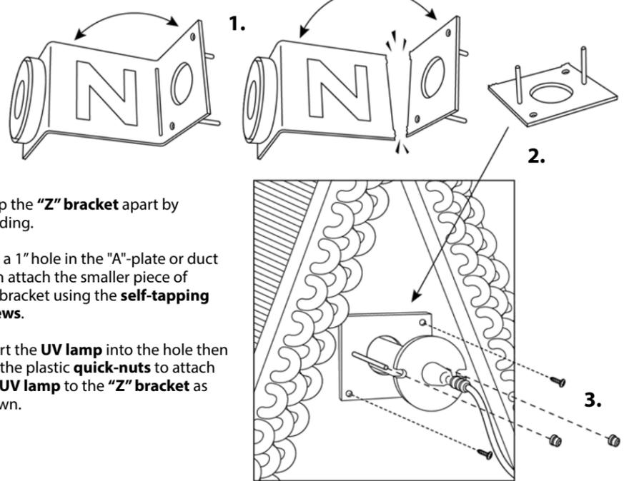
1. Snap the "**Z**" bracket apart by bending.
