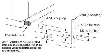
On horizontal units, a PVC stub or stainless steel tube is provided for condensate drain piping connection. An external trap is required (see below). If a vent is necessary, an open stand pipe may be applied to a tee in the field-installed condensate piping.
