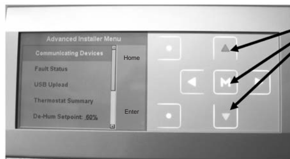
FIGURE 66 IN THE ADVANCED INSTALLER MENU SELECT COMMUNICATING DEVICES .
