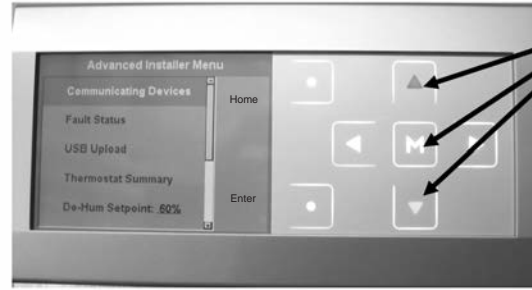
FIGURE 61 NAVIGATING TO COMMUNICATING DEVICES AND SELECT.
