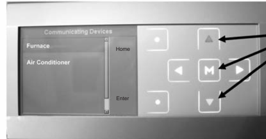
FIGURE 62 NAVIGATE TO FURNACE AND SELECT.
