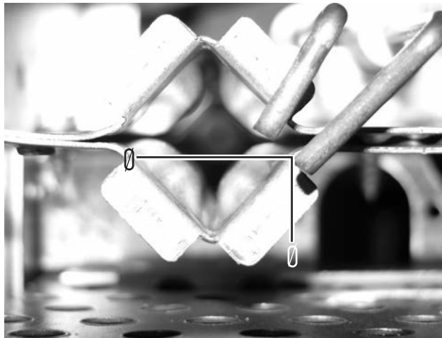
FIGURE 41 OPTIMUM IGNITOR LOCATION
