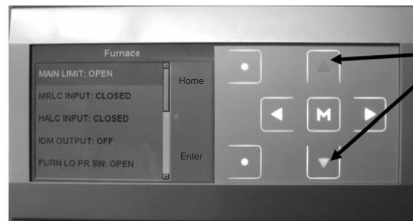
FIGURE 64 NAVIGATE THE USER MENUS USING UP AND DOWN ARROW KEYS.
