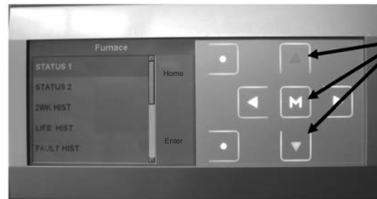
FIGURE 63 NAVIGATE TO DESIRED USER MENU AND SELECT.
