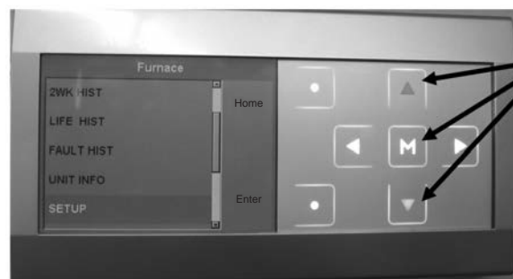
FIGURE 68 SELECT SETUP FROM THE LIST OF FURNACE MENUS.
