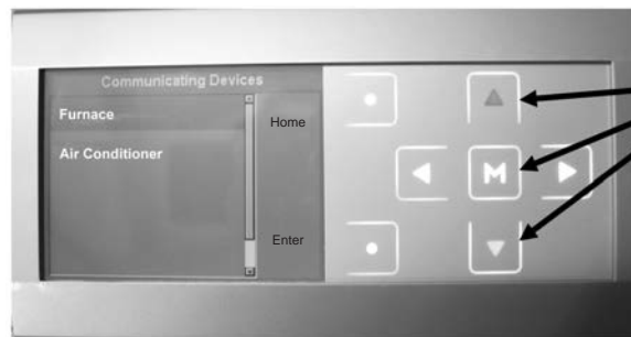
FIGURE 67 SELECT FURNACE FROM THE LIST OF COMMUNICATING DEVICES .
