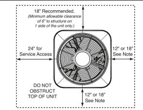
**NOTE:** Units require full perimeter clearances. Installer must maintain 18" between two units.
