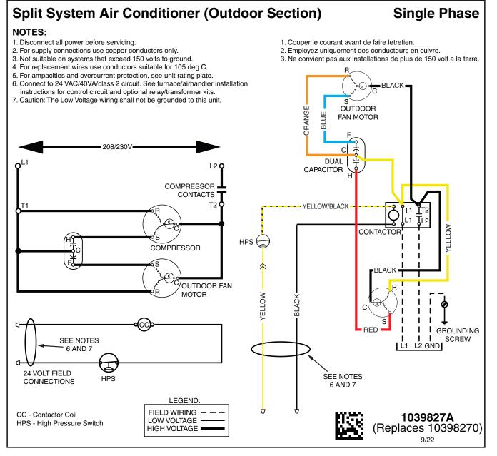
Figure 5. Wiring Diagram for RSA3ME4M1SN (3, 3.5, & 4 Ton Units)
