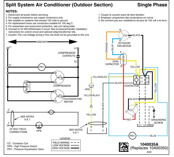
Figure 4. Wiring Diagram for RSA3ME4M1RN (2 & 2.5 Ton Units)
