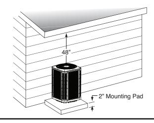
**Figure 1. Clearance Requirements**
