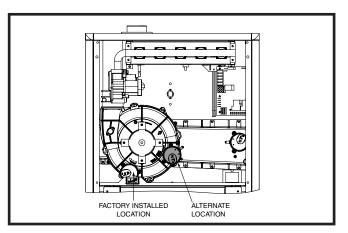
Figure 26. Alternate Pressure Switch Location
