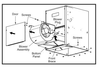
Figure 22. Bottom Panel Removal
