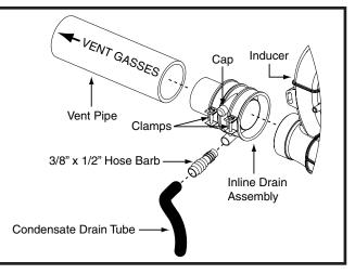
Figure 29. Inline Drain Assembly
