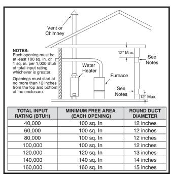
Figure 2. Combustion Air Drawn from Inside
