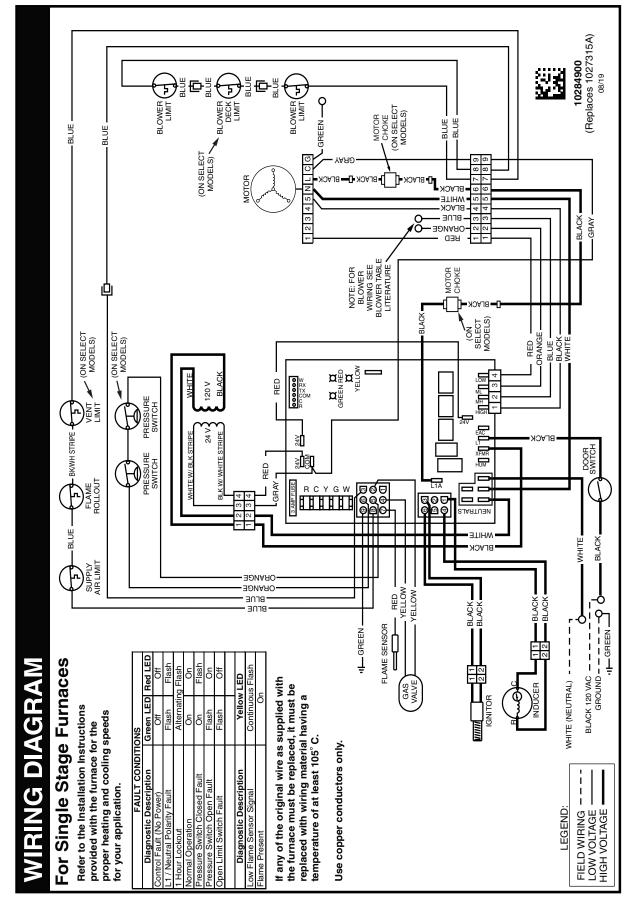
Figure 46. MG3P with Emerson Control Board Wiring Diagram
