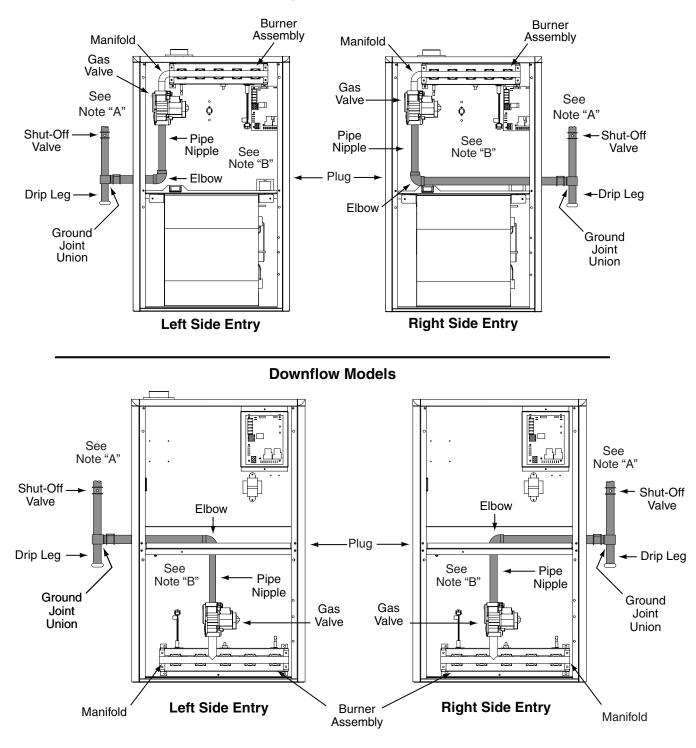
NOTE A: Consult local codes for Shut-Off Valve location requirements NOTE B: Inducer assembly omitted for clarity of pipe installatio
