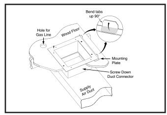
Figure 18. Screw-Down Duct Connector
