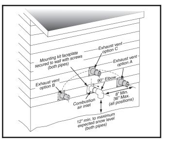
Figure 7. Inlet & Exhaust Pipe Clearances
