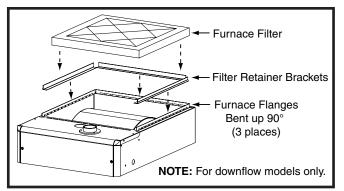
Figure 32. Filter Retainer Brackets
