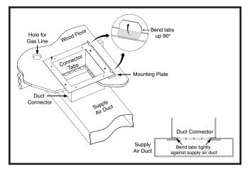
Figure 14. Duct Connector Installed
