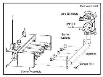
Figure 37. Burner & Manifold Assembly
