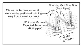
Figure 10. Vertical Vent Termination
