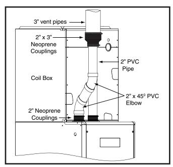
Figure 34. Alternate vent Pipe Installation
