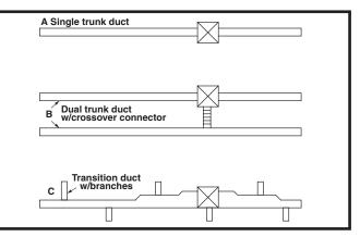
Figure 11. Typical Supply Duct System
