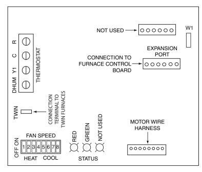
Figure 51. Two-Stage Fixed Speed Motor Control Board
