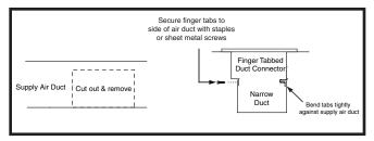
Figure 17. Narrow Air Ducts - Option 2
