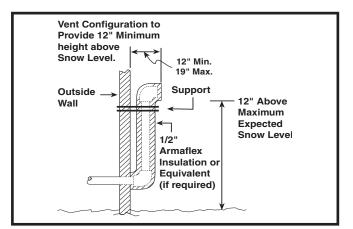
Figure 9. Alternate Horizontal Vent Installation
