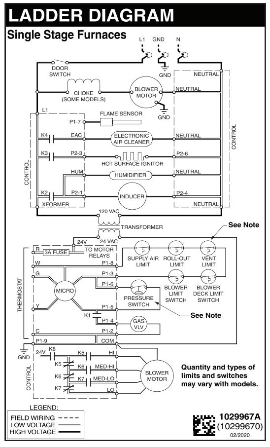
Figure 48. MG3P with Emerson Control Board Ladder Diagram
