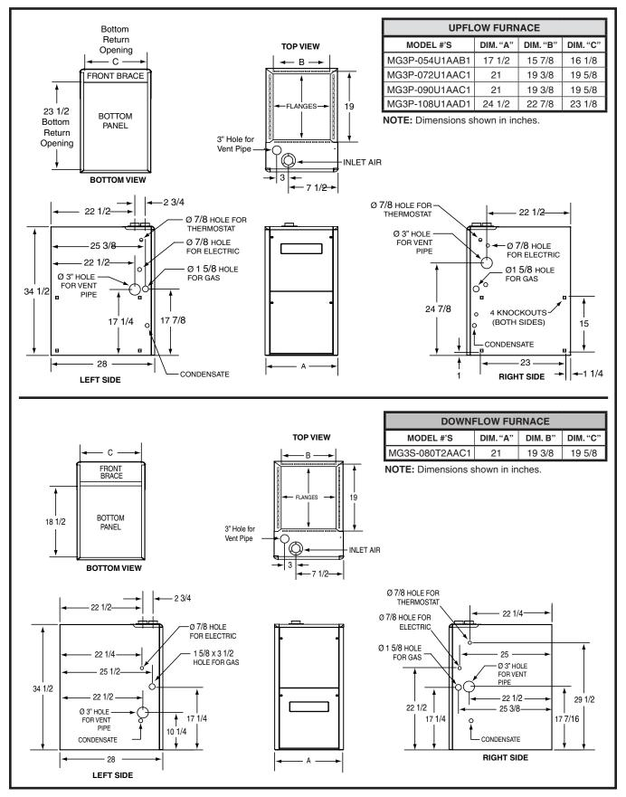
Figure 44. Furnace Dimensions
