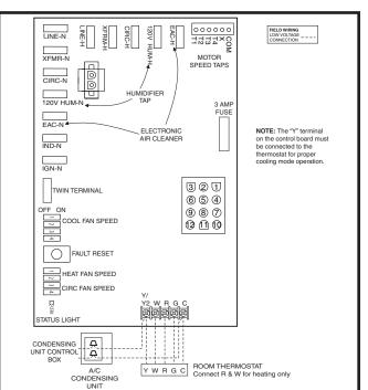
Figure 43. Emerson Low Voltage Field, Fourwire Heating/Cooling Applications
