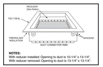
Figure 12. Duct Connector
