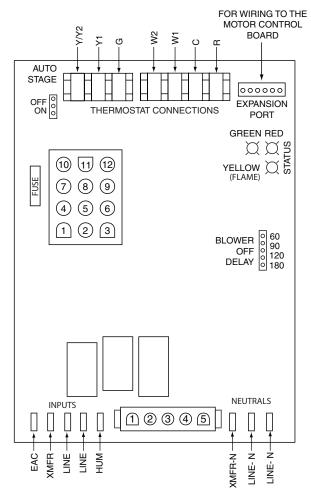
Figure 52. Two-Stage Furnace Control Board
