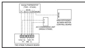
Figure 39. Wiring Configuration 2
