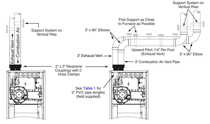
Figure 53. MG3P Horizontal & Vertical Venting
