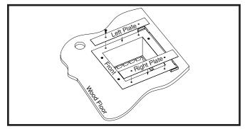
Figure 15. Duct Connector Side Plates
