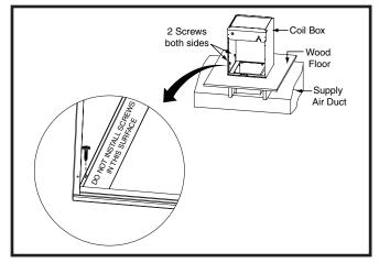
Figure 20. A/C Coil Box Installation
