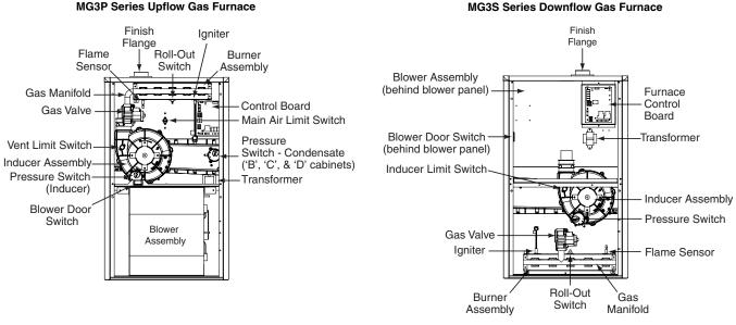
Figure 57. MG3(P,S) Component Locations
