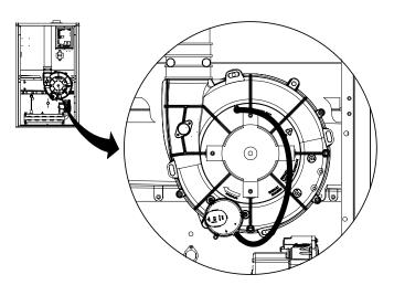
Figure 15. Pressure Switch Tubing for Downflow Furnaces Models J951X054D, J951X072D, & J951X090D
