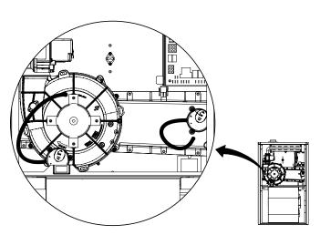
Figure 14. Pressure Switch Tubing for Upflow Furnaces Models J951X038U, J951X054U, J951X072U, J951X090U, J951X108U, & J951X120U
