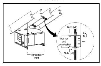
Figure 12. J951X\*U Horizontally Suspended in an Attic
