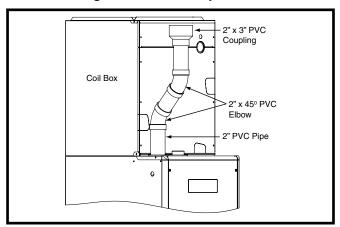
Figure 20. Optional PVC Pipe Installation
