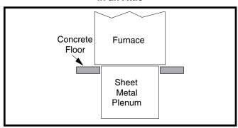
Figure 13. Furnace on a Concrete Slab
