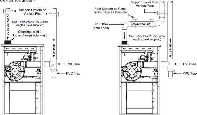
Figure 33. Horizontal & Vertical Venting
