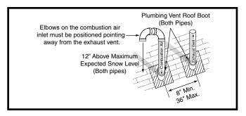
**Figure 10. Vertical Vent Termination**
