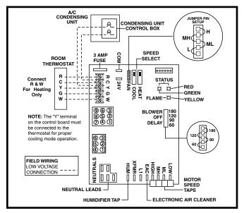
Figure 26. Low Voltage Field, Four-wire Heating/Cooling Applications
