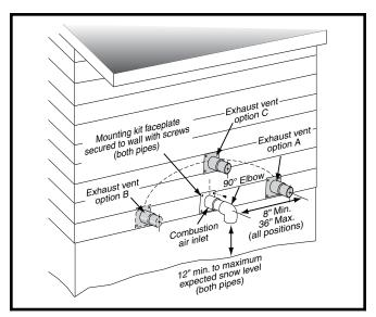
Figure 7. Inlet & Exhaust Pipe Clearances
