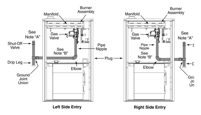
Figure 23. Typical Gas Connections - Upflow Models
