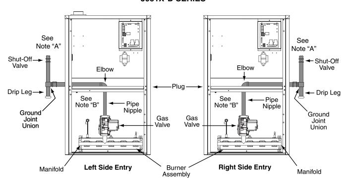
NOTE A: Consult local codes for Shut-Off Valve location requirements NOTE B: Inducer assembly omitted for clarity of pipe installatio
