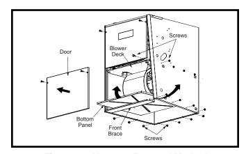
Figure 22. Alternate Removal Method
