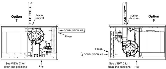
Figure 35. Venting Options for Horizontal Installations (J951X\*U Series)
