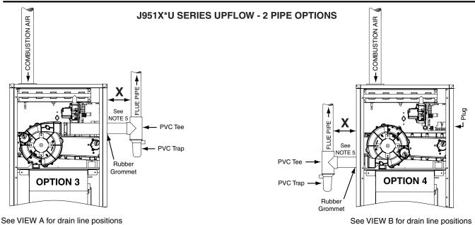
Figure 34. Venting Options for Upflow Installations (J951X\*U Series)
