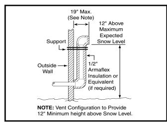
Figure 9. Alternate Horizontal Vent Installation
