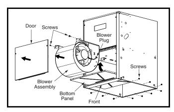
Figure 21. Bottom Panel Removal
