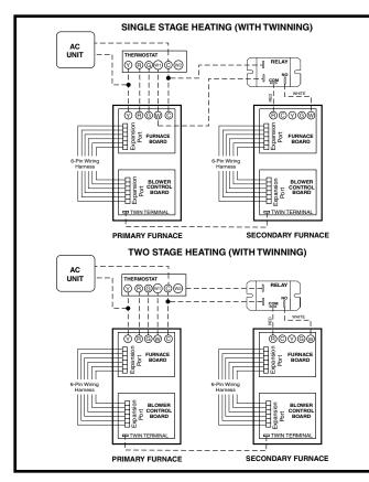
Figure 27. Single & Two Stage Twinning
