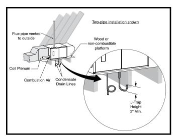
Figure 11. J951X\*U Horizontal installation on a Platform
