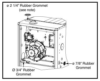
Figure 18. Rubber Grommets
