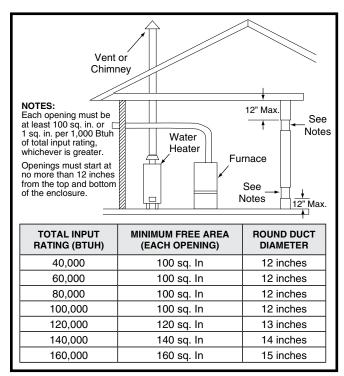
Figure 2. Combustion Air Drawn from Inside
