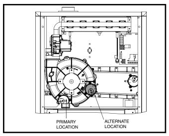
Figure 16. Alternate Pressure Switch Location
