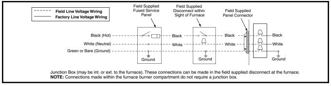
Figure 25. Line Voltage Field Wiring
