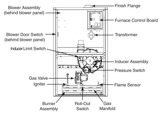
Figure 38. J951X\*D Component Locations
