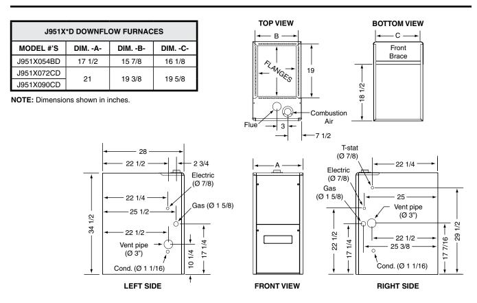
Figure 30. J951X\*D Cabinet Dimensions
