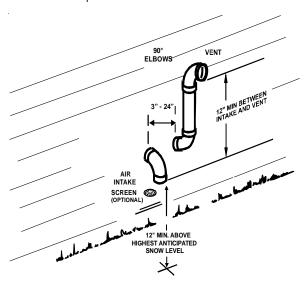
Alternate Horizontal Vent Termination (Dual Pipe)
