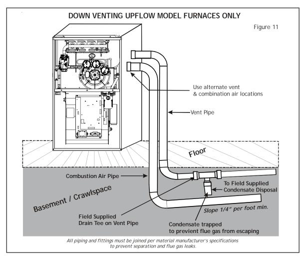
NOTE: Terminate both pipes in the same pressure zone (same side of roof, no major obstacles between pipes, etc.).
