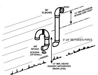
Combustion Air Intake may also be snorkeled to obtain 12" min ground clearance.
