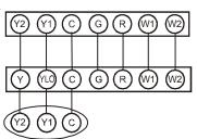
Remote Condensing Unit (Two-Stage Cooling) Furnace
