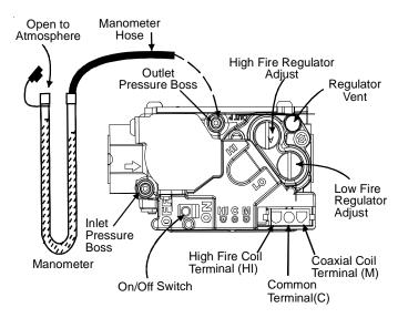
White-Rodgers Model 36J54 Connected to Manometer Figure 33B
