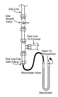
Measuring Inlet Gas Pressure (Alt. Method) Figure 34
