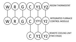
THERMOSTAT - SINGLE-STAGE HEATING WITH TWO-STAGE
