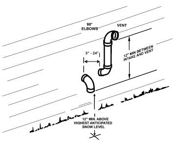
ALTERNATE HORIZONTAL VENT TERMINATION (DUAL PIPE)
