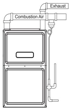
TEE INSTALLATION IN INTAKE PIPE FIGURE 8
