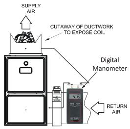
CHECKING STATIC PRESSURE (80% FURNACE SHOWN, 90% SIMILAR) FIGURE 42
