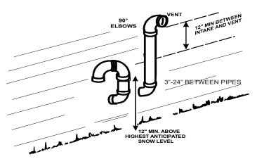
COMBUSTION AIR INTAKE MAY ALSO BE SNORKELED TO OBTAIN 12" MIN GROUND CLEARANCE.
