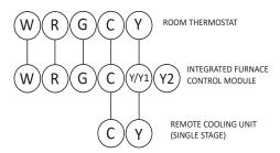
THERMOSTAT - SINGLE-STAGE HEATING WITH SINGLE-STAGE COOLING FIGURE 34
