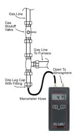
MEASURING INLET GAS PRESSURE (ALT. METHOD)
