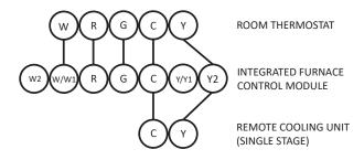
Thermostat - Single -Stage Heating with Single-Stage Cooling **NOTE**: To apply a single-stage Heating Thermostat, the staging option *must* be set on single-stage.
