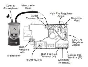
White-Rogers Model 36J54 Connected to Manometer Figure 20B
