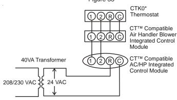
System Wiring using Two-Wires between Air Handler and AC/ HP and Four-Wires between Air Handler and Thermostat Figure 24
