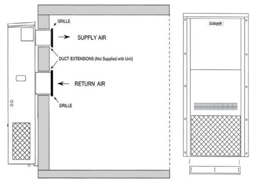
For units with electric heat, a one inch clearance is required around the duct extensions. The duct extensions must be constructed of galvanized steel with a minimum thickness of .019" as per the NFPA standards 90A & 90B.
