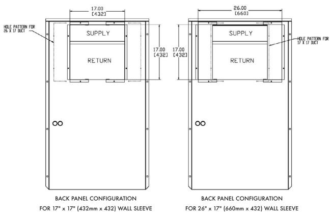
Figure 6. Back Panel Configuration for WalPac II AVPA12 Air Conditioners
