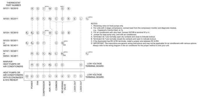
Figure 9b. Thermostat Connection Diagram
