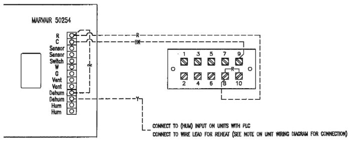
Figure 9a. Humidistat (P/N 50254) Wiring to a WalPac Air Conditioner with Reheat.
