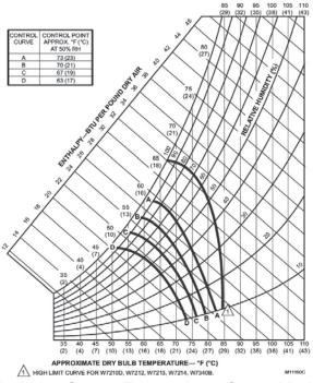
Figure 3. Enthalpy Sensor Temperature Control Points
