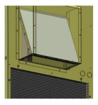
HVESA models with the vertical economizer utilize external gravityoperated exhaust outlet dampers located on each side of the unit. The dampers are covered by a hood to exhaust the air in upward direction, away from the economizer inlet. The hood also prevents rain, debris and pests from entering the unit.
