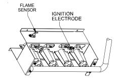
Flame Sensor and Ignition Electrode Location
