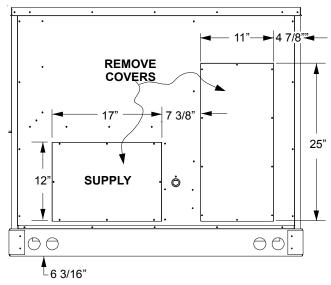
**Horizontal Discharge Duct Connections**
