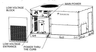
**Power and Low Voltage Block Connections**
