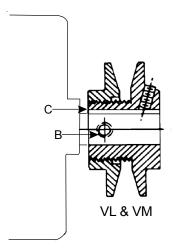
**NOTE:** Do **NOT** operate sheave with flange projecting beyond the hub end.
