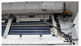
Fig. 32 - Connect the multi-function board
