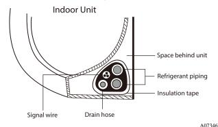
**Fig. 26 – Bundle drain hose, refrigerant pipes, & signal cable NOTE**: For applications where gravity cannot be used for drainage, a condensate pump accessory is available. Consult the condensate pump Installation Instructions for more information.
