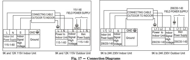
Notes: 1. Do not use thermostat wire for any connection between indoor and outdoor units. 2. All connections between indoor and outdoor units must be as shown. The connections are sensitive to polarity and will result in a fault code.
