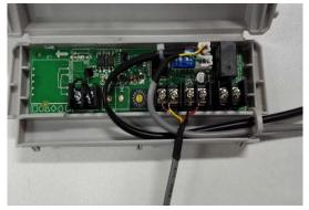
Fig. 30 – Connect the cable to the board
