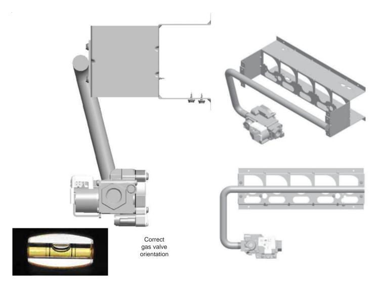
When installing a replacement gas valve on a modulating furnace, special attention must be given to gas valve positioning.
