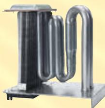
The award-winning design of the primary heat exchanger in the Goodman brand GMH8/GDH8 is unique. It's constructed from tubular aluminized-steel and formed into a dual diameter configuration. Furthermore, the use of wrinkle-bend technology results in an extremely durable heat exchanger. A heat exchanger often is considered the essential component of any gas furnace. This combination offers one of the best levels of reliability, durability, and efficiency you'll find within the Goodman brand.
