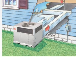
Packaged Gas Heating/Electric Cooling System
